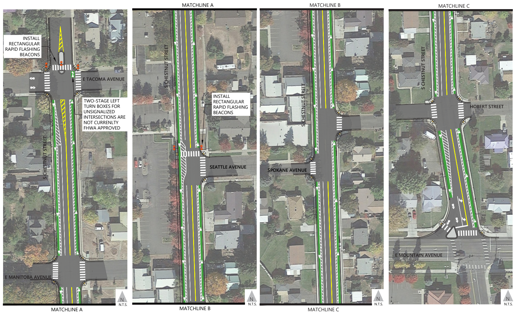
Figure 11 - Conceptual Design of Buffered Bike Lanes Along S Chestnut Street, Including RRFBs and Crossing Islands
