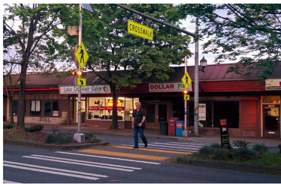
Level B: Rapid Rectangular Flashing Beacons
