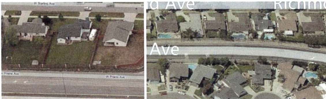
Figure 15.420.030(D)(1). Examples of reverse frontage lots that back up to collectors and arterial streets (note fences lining the street) (images courtesy of Bing maps).
